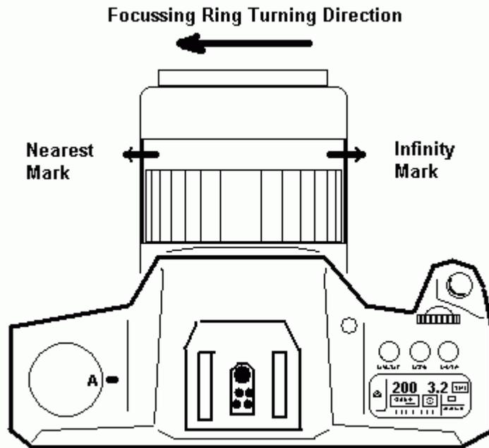
(2) When handling focusing at big aperture size (e.g. f/1.4) the depth of field is so thin such that very tiny further movement of the focusing ring after you get the indicator might induce a significant off-focus result. Hence it is good to practise well a technique of stop turning the focusing ring once the indicator shines.
